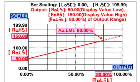
**Fine zero & span adjustment:**
