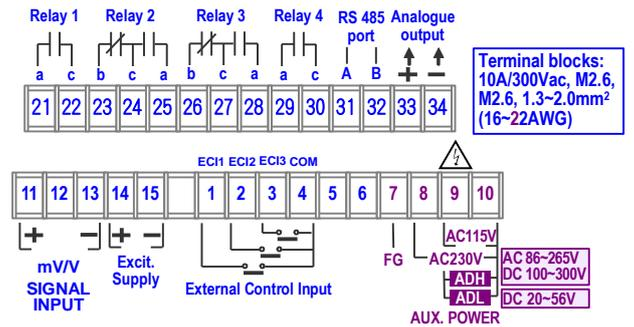
Please check the voltage of power supplied first, and then connect to the specified terminals. It is recommended that power supplied to the meter be protected by a fuse or circuit breaker.
