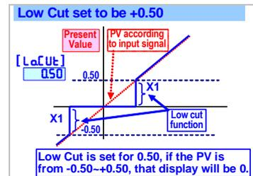
2. If set the negative value (X2) here to display "X2" which is expressed to be low-cut the PV that it's under the X2 setting value;
