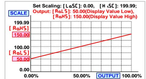
The range between [RaHS] and [RaLS] should be over 20% of span at least; otherwise, it will be got less resolution of analogue output.
